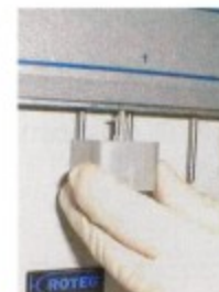
6. insert cup holder in measurement position after mixing of reagents and sample
